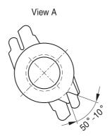
Hole arrangement View in mounting direction
