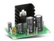
This small amplifier is constructed around the TDA2003 IC, capable of delivering 4Wrms at 40hms. The IC is completely thermally and short-circuit protected. A conventional direct current can be connected as supply.
