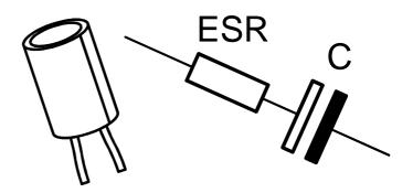
No capacitor is ideal of course, the detailed equivalent circuit of a typical capacitor is very complex. For many electrolytic capacitors however, the most important parameters regarding the capacitor's performance is the capacitance and the ESR.
