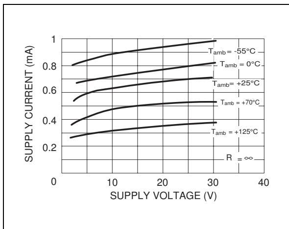
**INPUT CURRENT versus SUPPLY VOLTAGE**
