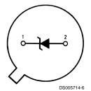
Pin 2 is electrically connected to case
