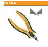
TR 20 M: Tool for a flush cut. The reduced head's dimension and its pointed shape, allow access to difficult to reach areas. Steel thickness 2.0 mm. Tool length 132mm. Safety clip for holding wire scraps securely after cutting available (order code TR 20 M A). Safety clip type AF.
