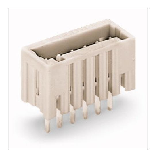
Printview: Male header (for PCBs); Straight solder pin 0.8 x 0.8 mm; 3-pole; Pin spacing 2.5 mm / 0.098 in; 100% protected against mismating; Vertical PCB mounting; with closed end - Item No.: 733-333
