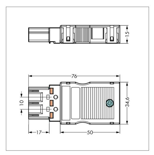
Printview: Plug; with strain relief housing; 3-pole; Pin spacing 10 mm / 0.394 in; 100% protected against mismating; Cable diameter 8 - 11.5 mm - Item No.: 770-113
