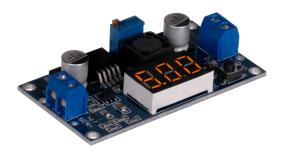
This is a voltage converter based on the DC-DC module LM2596S. The voltage can be adjusted by the potentiometer with an accuracy of  $\pm$  0.1 V (DC). The integrated segment display can additionally be switched between the input and the output voltage via the button.
