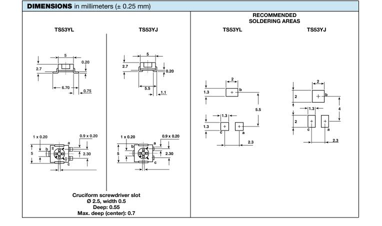
The TS53 trimming potentiometer has been designed for surface mount applications and offers volumetric efficiency (5 mm x 5 mm x 2.7 mm) with high performance and stability.
