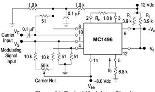
Figure 24. Typical Modulator Circuit
