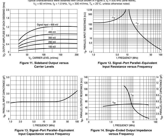
Typical characteristics were obtained with circuit shown in Figure 5,  $f_{\rm C}$  = 500 kHz (sine wave),
