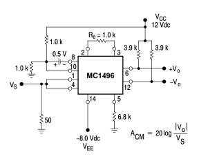
Figure 9. Common Mode Gain
