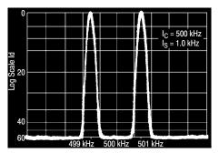
Figure 2. Suppressed Carrier Spectrum
