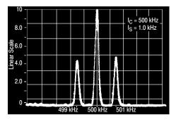
Figure 4. Amplitude–Modulation Spectrum
