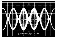
Figure 1. Suppressed Carrier Output Waveform
