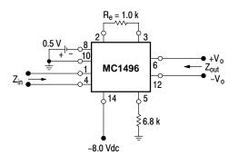
**NOTE:** Shielding of input and output leads may be needed to properly perform these tests.
