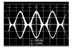
Figure 3. Amplitude Modulation Output Waveform
