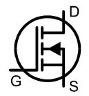
the bias of the gate-source voltage is always positive (For N-Channel types). The other (rarer) type of MOSFET is the Depletion Mode type which is described in a later section.
