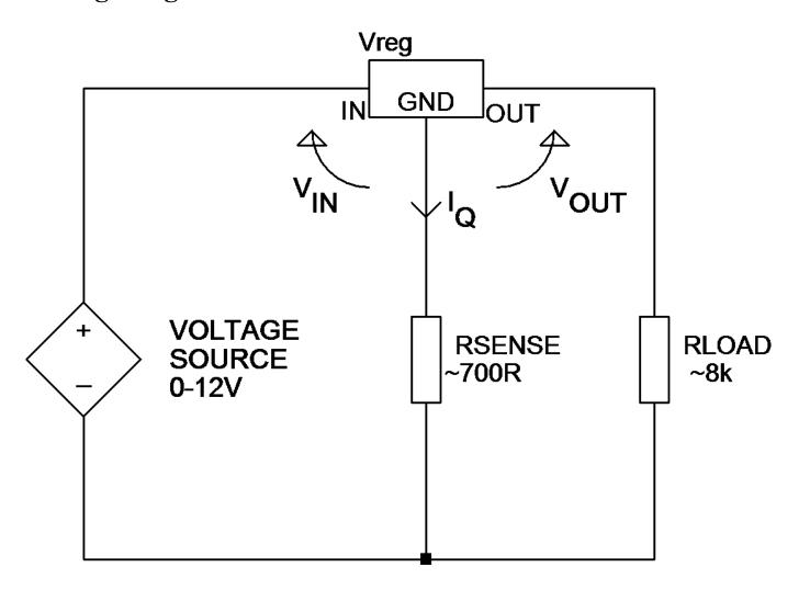
The test circuit shown here is used for the analysis of voltage regulators (positive regulators in this example). Note that the range of regulator voltages supported will depend on the quiescent current ( $I_Q$ ). A higher quiescent current will cause more voltage to be dropped across the sense resistor and yield less voltage for the regulator itself.
