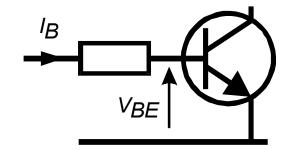
VBE=0.703V at IB=5.00mA **-**|k This example shows an NPN base-emitter voltage ( $V_{BE}$ ) of 0.703V for a base test current ( $I_B$ ) of 5mA.
