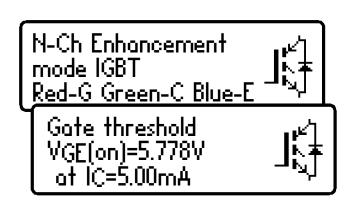
Similar to the MOSFET analysis, the gate threshold is the voltage between the gate and emitter that causes the device to start conducting (between the collector and emitter). The **DCA Pro** determines that conduction has started if the collector current has reached 5.0mA.
