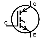
It combines the input characteristics of a MOSFET with the output characteristics of a Bipolar Junction Transistor.
