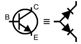
junction represents the base terminal. This is normal for situations where the current gain is so low that it is immeasurable at the test currents used by the **DCA Pro**.
