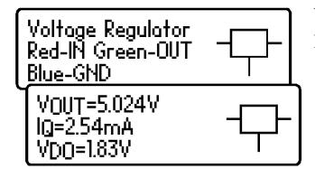
When a regulator is identified, its pinout, output voltage, quiescent current consumption and drop-out voltage are displayed.
