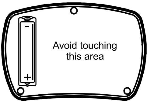
We recommend that the battery is replaced with a high quality battery equivalent to an **Alkaline AAA**, LR03 or MN2400 (1.5V). Replacement Alkaline AAA batteries are available from many retail outlets.
