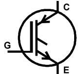
Depletion mode IGBTs are characterised by the fact that current can flow between the collector and emitter when there is zero voltage across the gate-emitter terminals.
