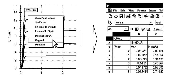
Pasting the data into a spreadsheet is an ideal way of documenting important test results.
