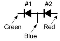
In the same way as the single diode analysis, the forward voltage for each diode is measured for a nominal test current of 5mA.
