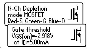
between its drain and source terminals even with a zero voltage applied across the gate and the source. The device can only be turned completely off by taking its gate significantly more negative than its source terminal, say –5V. It is this characteristic that makes them so similar to conventional JFETs.
