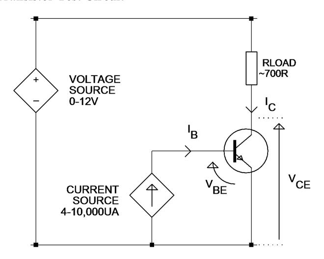
Example shown is for an NPN transistor. Polarities are reversed for PNP devices
