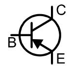
variations are automatically identified by the *DCA Pro* and their schematic symbol display on the screen. Both NPN and PNP types are supported.
