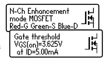
The (on) gate threshold voltage is the gate-source voltage at which conduction between the source and drain starts. The *DCA Pro* determines that drain-source conduction has started when it reaches a current of 5.00mA, this is confirmed on the display.
