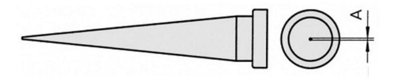
Soldering tip of the LT series for soldering irons WP80 / WSP80 / MPR80 / FE75
