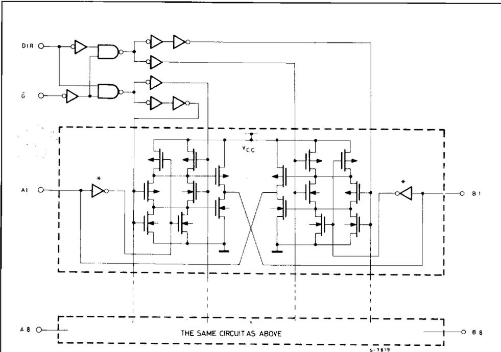
NOTE: IN CASE OF HCT245 OR HCT643, INPUT INVERTERS MARKED \* AT A BUS OR AT B BUS ARE ELIMINATED RESPECTIVELY.
