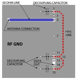
Note: Dotted elements must be placed on component side ( PCB side opposite to ground layer ). Note: This is a general layout, in some modules it could be slightly different (e.g. pin 1 and/or pin 15 not mounted)
