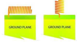
can be achieved by spreading or compressing the coil. If the coil is wound tightly enough, it may be shorter than one-tenth of a wavelength.
