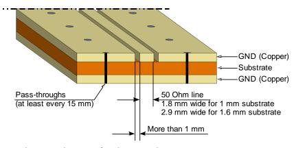
Note: the dimensions in the picture above are referred to a FR4 substrate PCB
