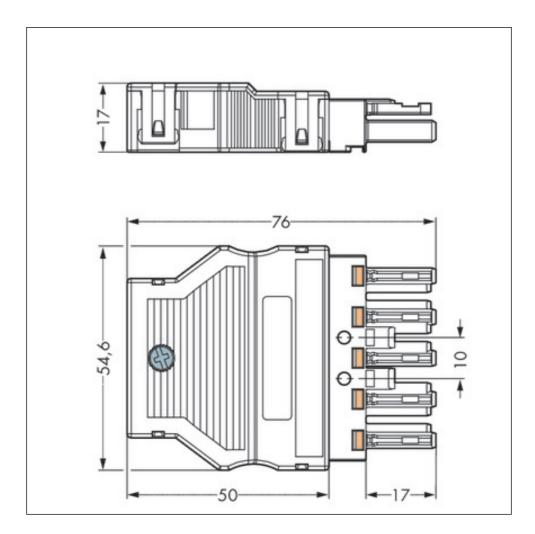
Printview: Socket; with strain relief housing; 5-pole; 100% protected against mismating; Cable diameter 9 - 13 mm; 1-conductor connection - Item No.: 770-325
