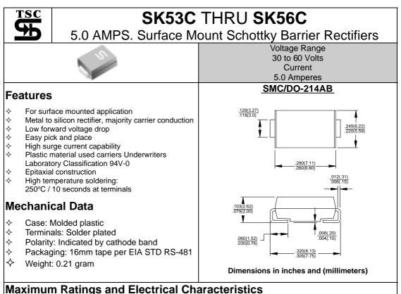
Rating at 25°C ambient temperature unless otherwise specified.
