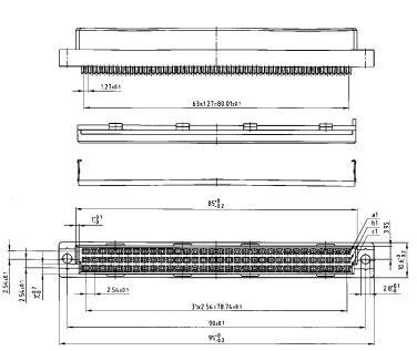
Female connector with strain relief
