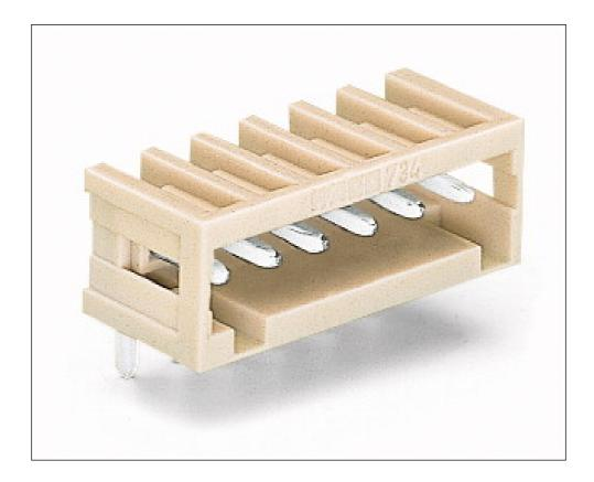
Printview: Male header (for PCBs); Angled solder pin 1 x 1 mm; 16-pole; Pin spacing 3.5 mm / 0.138 in; 100% protected against mismating; with closed end; Horizontal PCB mounting - Item No.: 734-176
